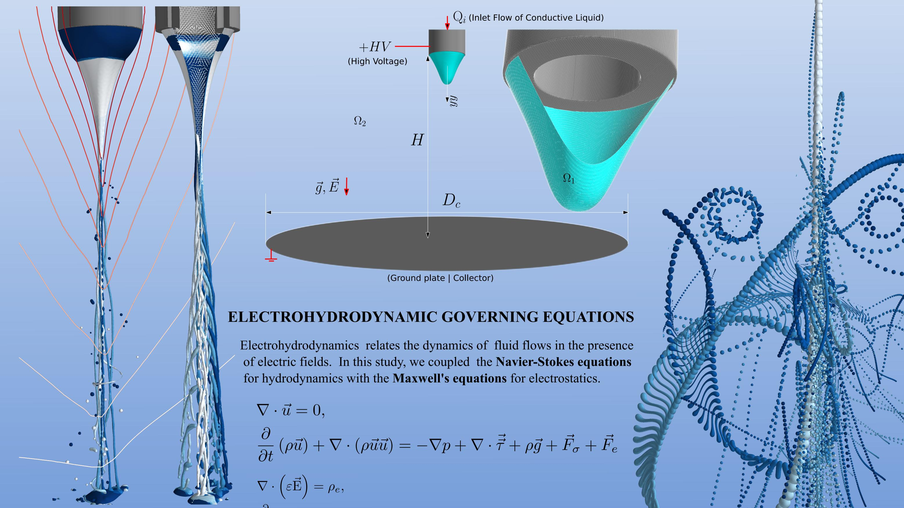
*blues: Liquid free-surface (colored by time)* reds: Field isolines of electric potential
